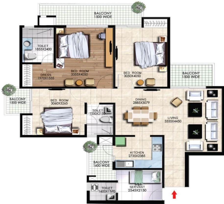
TYPICAL UNIT PLAN 3 BED + 3 TOI + SERVANT Carpet Area: 1010.192 sq. ft. Built-up Area: 1342.258 sq. ft. Saleable Area: 1670 sq. ft.
